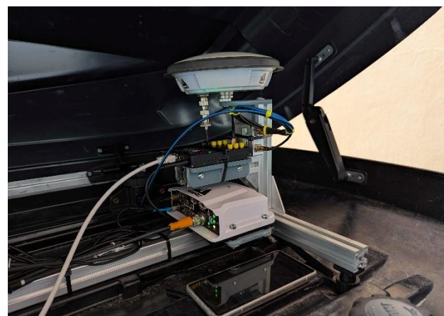
Figure 5. Detail of the GNSS receiver area of the aluminum structure at the back of the car.
