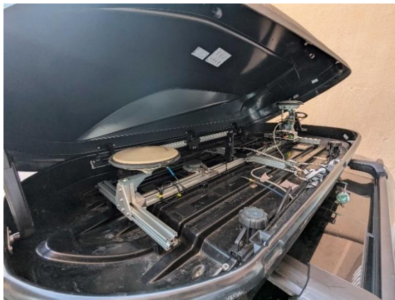
Figure 4. Extruded aluminum structure with equipment installed on top.
